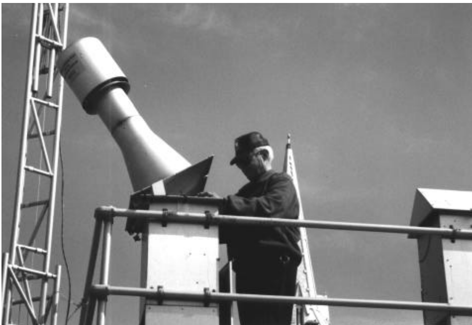
An air quality technician with the state's air pollution control division services an air monitoring device atop the air monitoring trailer in Burlington.
