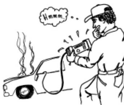
Using a scan tool a technician can quickly diagnose engine problems.
