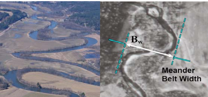
Figure 3. River meanders like those on the Lamoille River are best viewed from the air (left). The meander belt width is measured as the lateral distance between the outermost bends of a meander, when a river is in "equilibrium" condition (right).
